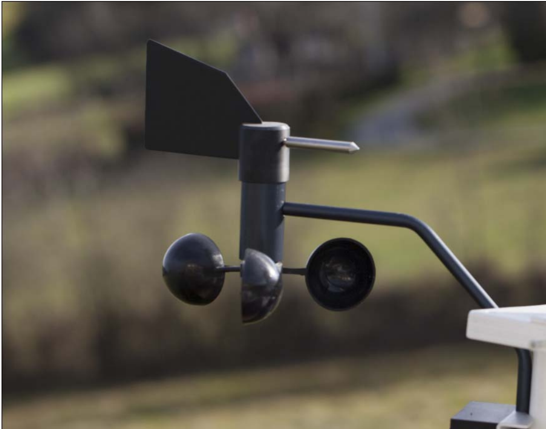
Fig. 91 Wind speed and Wind direction sensor
