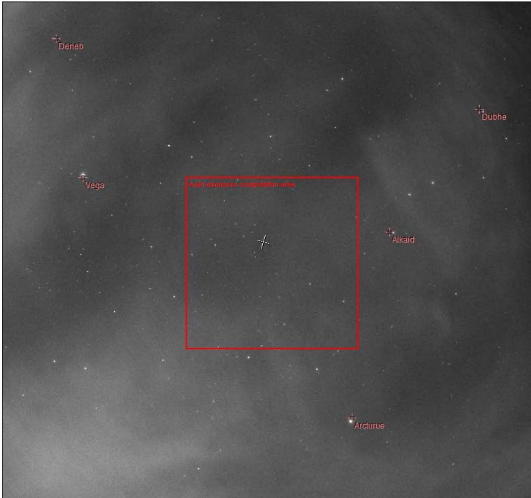
Fig. 51 If the computing area for auto exposure is set to 512x512 image center, this shape is drawn to show where the bounds of this area are located.
