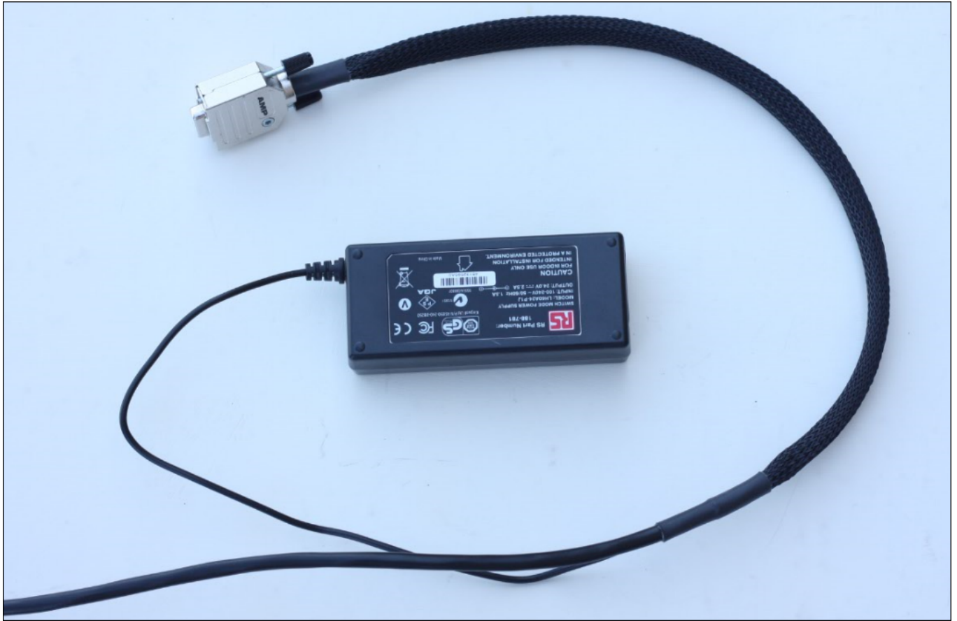
Fig. 11 RS232 connector and 24V 2.5A power
