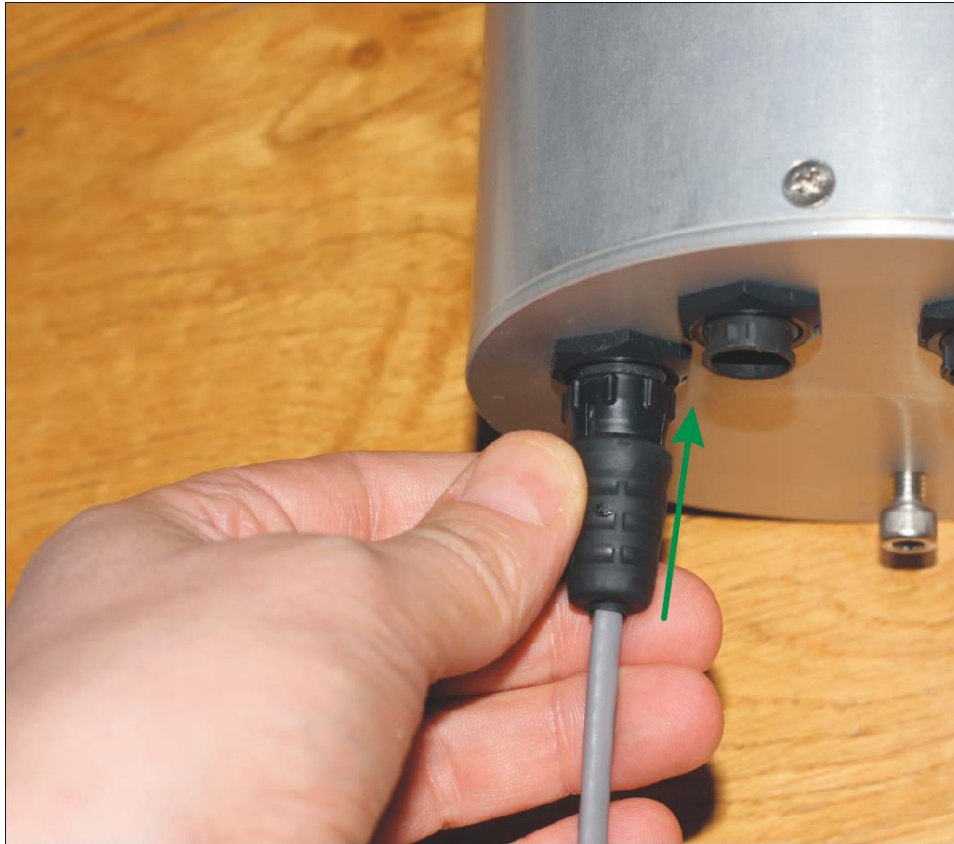
Fig. 7 Push the connector straight
