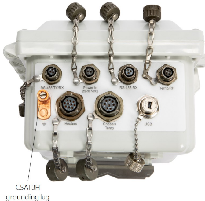
Figure 6-12. Grounding lug and connectors on bottom of CSAT3H heater controller box
