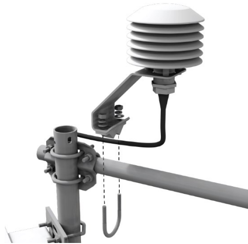
Figure 6-5. Mounting the temperature/relative humidity probe
